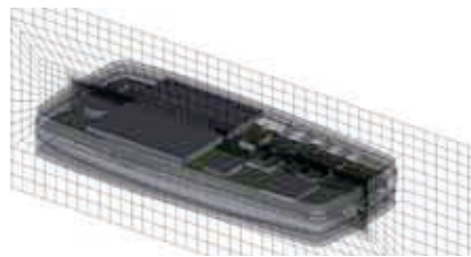
Multi-level hex-dominant mesh of cell phone assembly; hanging-node mesh resolves small geometric details.
