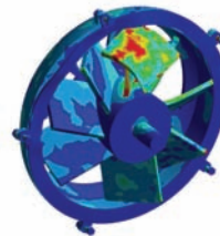
Blade-off containment demonstrating failure of bonded connection and subsequent complex body interactions (contact)
