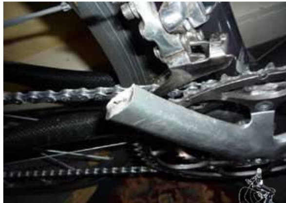
Bicycle crank shaft broken due to fatigue
