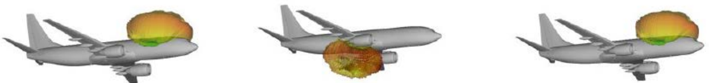
Figure 3. UHF Blade antenna patterns due to different locations.
